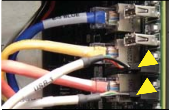
Figure 8. Remove USB Module Cables From CPU Board
