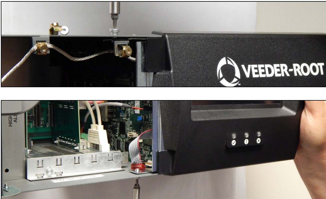
Figure 7. Remove Top And Bottom Display Door Hinge Screws
