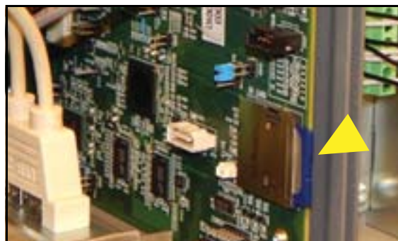
Figure 24. Locating SD Card On CPU Board
