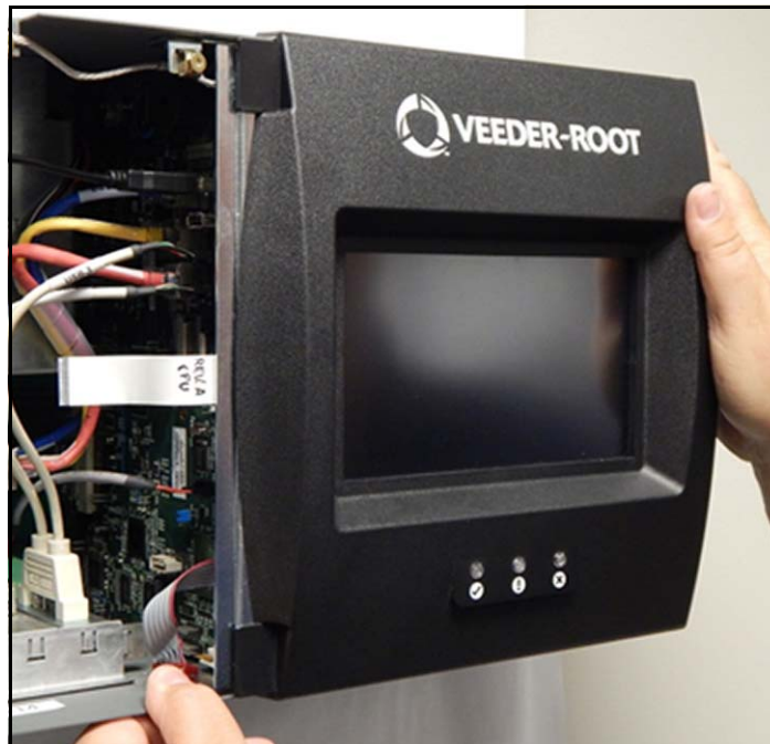
Figure 21. Install The New TLS-450PLUS Display Door
