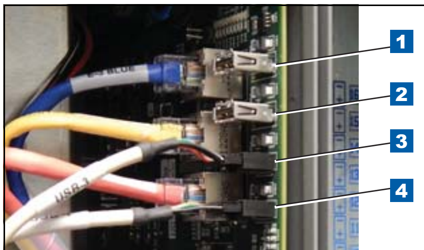
Figure 19. Connect USB Module Cables
