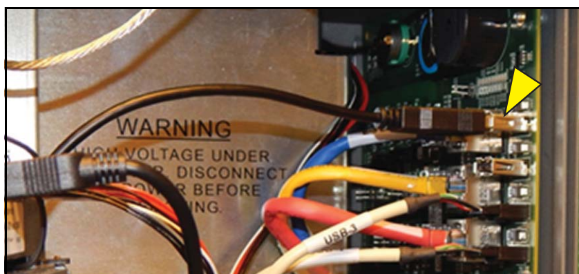
Figure 20. Connect Optional Printer USB Cable
