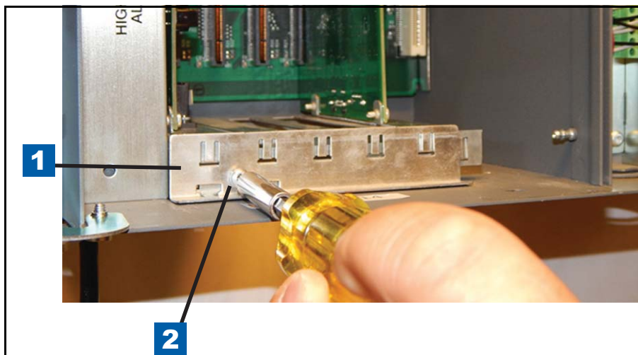
Figure 10. Removing Comm Module Clamp
