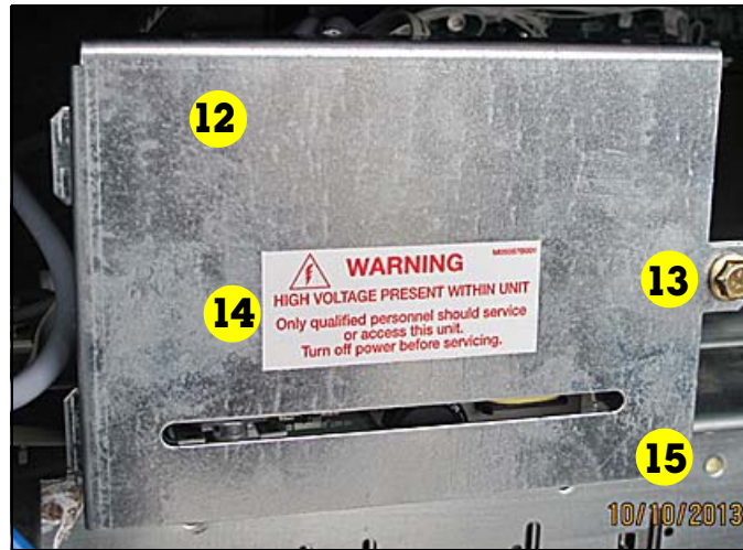
Figure 10. Attach The VaporTEK Controller Safety Cover
