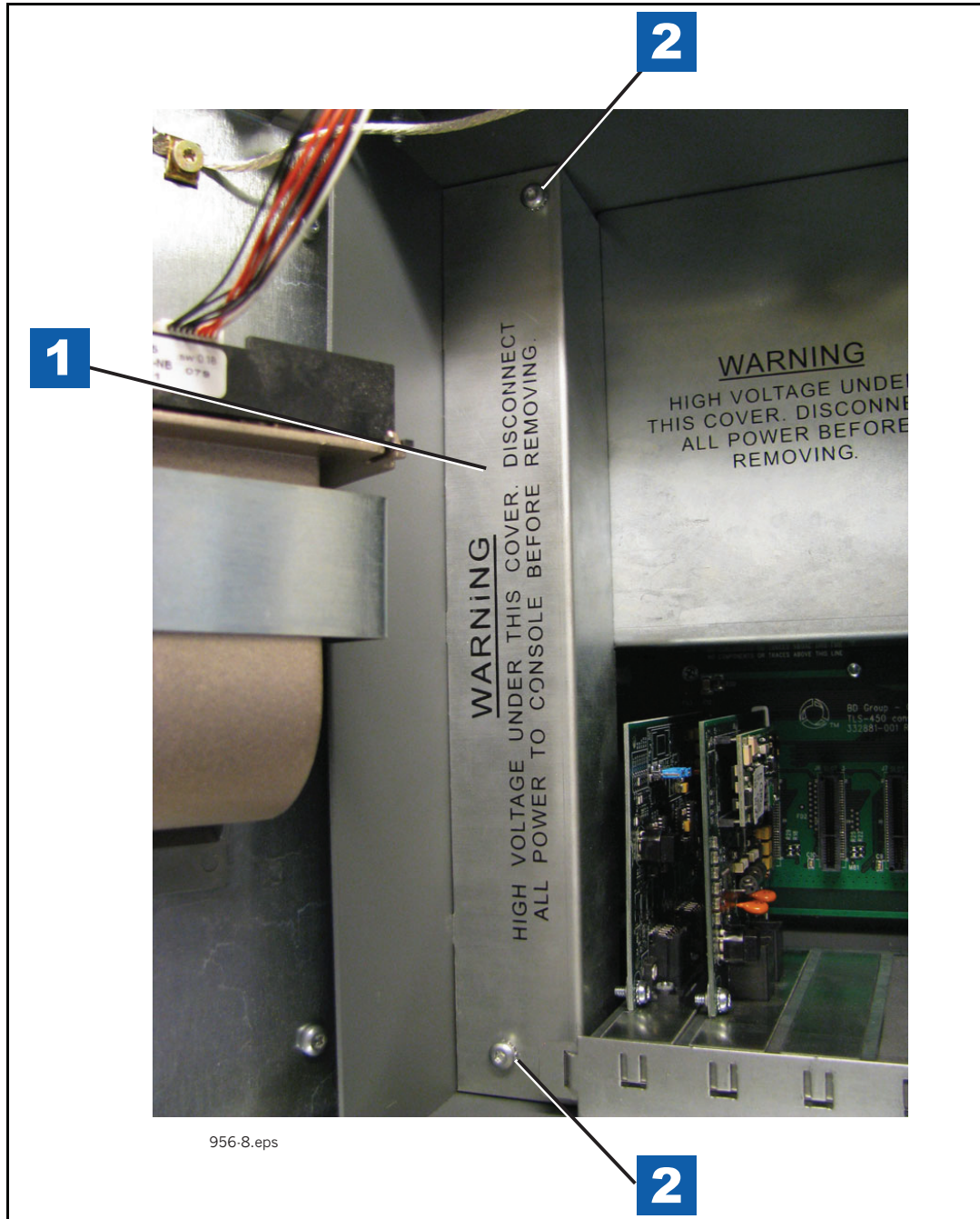
Figure 6. Remove AC Channel cover
