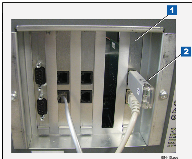
Figure 1. USB/Ethernet board - V-R thumb drive port
